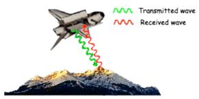
When radar bounces off the ground, only some of the signal gets back to where it started. Much of the signal scatters in other directions. How much of the signal scatters depends on how smooth or rough the surface
